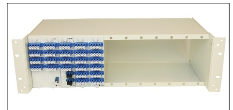
3U modular panel with CWDM modules
